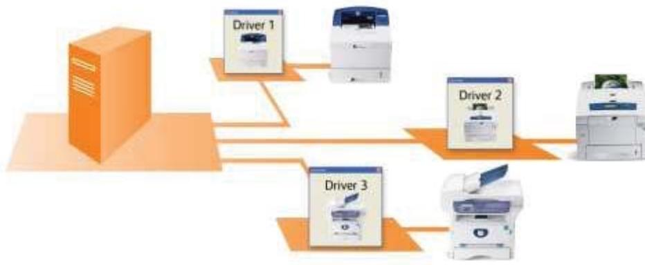
*The traditional one printer: one driver model significantly increases IT’s driver management and support burden, and is frequently a source for driver conflicts on network print servers. Most “universal” print drivers are proprietary and support relatively few devices on the typical network, doing little to resolve this issue.*
